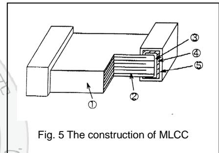
Fig. 5 The construction of MLCC
