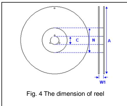
Fig. 4 The dimension of reel
