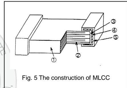
Fig. 5 The construction of MLCC
