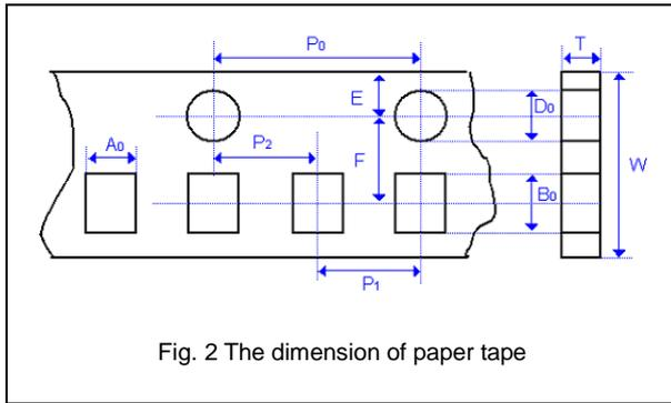
Fig. 2 The dimension of paper tape
